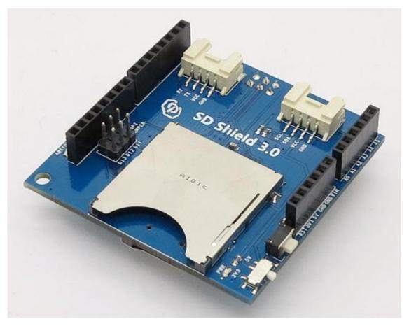
SD Shield 3.0 is a break out board for standard SD and TF card. It is compatible with 5V and 3.3V Arduino mainboards, Arduino-compatible boards and Arduino mainboards that SPI is on ICSP instead on pin D11~13 such as Leonardo.
