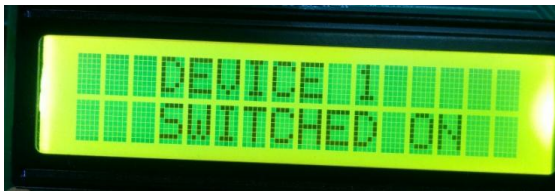
Fig.10. Status of Load-1 Displaying On LCD at Transmission End Module.
