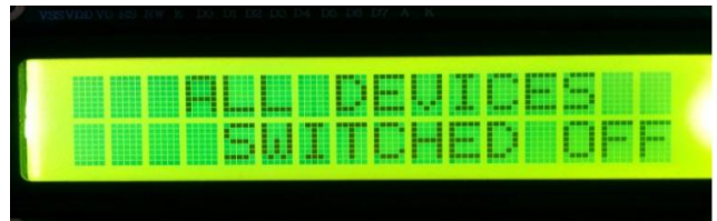
Fig. 5. lcd display at transmitting end when all loads are switched off.
