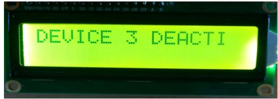
Fig.12. Status of Load-3 Displaying On LCD at Transmission End Module.
