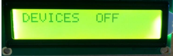
Fig. 7. lcd display at receiving end when all the loads are in off state.
