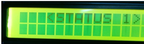
Fig.9. Display of LCD to Find Status of Load-1 at Transmission End Module.
