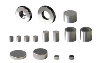
All NdFeB magnets should have some form of protective coating to minimise and ideally prevent corrosion. Uncoated is not advised. The default / standard protective coating is Ni–Cu–Ni plating. Other coatings/finishes exist (over 40 finishes are currently available). Where maximum corrosion resistance is required for NdFeB, consider using the increased corrosion resistance range of NdFeB alloys.
