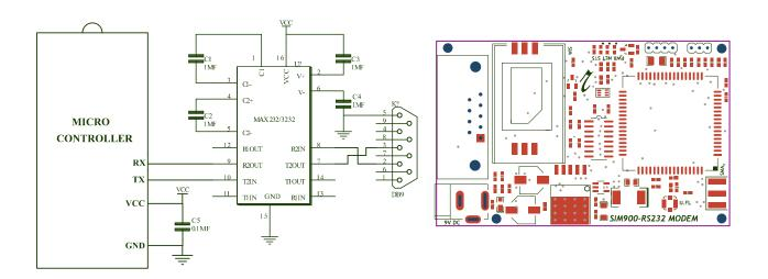
Fig:3 GSM Modem Interfacing with Microcontroller
