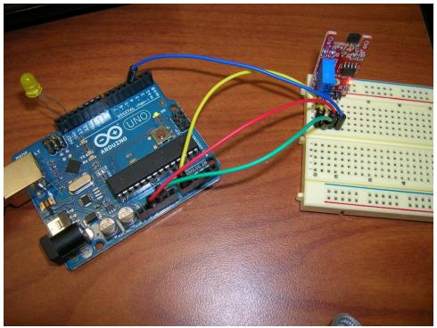
The yellow wire is connected to A0 on the sensor, and A0 on the Arduino. The green wire is connected to G on the sensor and GND on the Arduino. The Red wire is connected to + on the sensor and 5V on the Arduino. The blue wire is connected to D0 on the sensor and Digital 3 on the Arduino. The LED has it's long prong in DIGITAL 13 and its short pin in GND.
