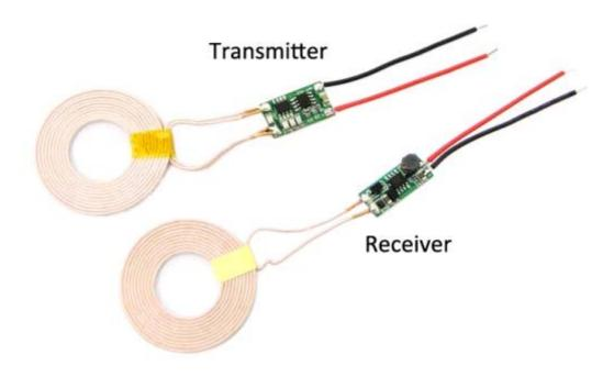
The Wireless Charging Module can be applied in electronic equipments in common use for close wireless charging or power supply. Consisted of a transmitter and insulation coil, it could serve as a replacement for the Wireless Power Supply with stable 5V output voltage and maximum 1.2A output current. Its small size and insulation coil is more suitable for using in wireless project.
