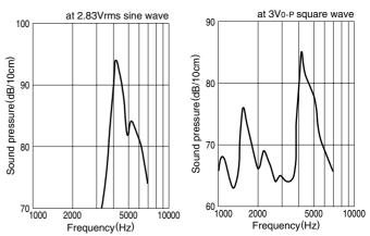
\* The frequency characteristic changes depending on the case shape and the installation method.
