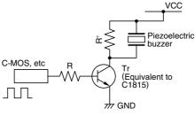
$^{\ast}$  Resistor to do charging and discharging to a piezoelectric element (Value of about 1k $\Omega$  is good efficiency).
