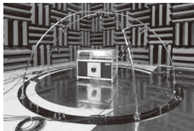
Noise characteristic measurement equipment
